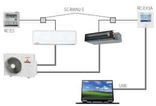
RC-EX 3A control can be controlled via computer by using a special software.
