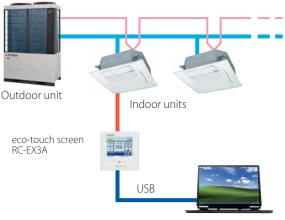
RC-EX 3A control can be controlled via computer by using a special software.
